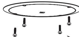
4 pcs - M4 x 38mm powder coated machine screws for attaching the metal grille to the baffle. (Included with MTC-RG6/8 grille.)
