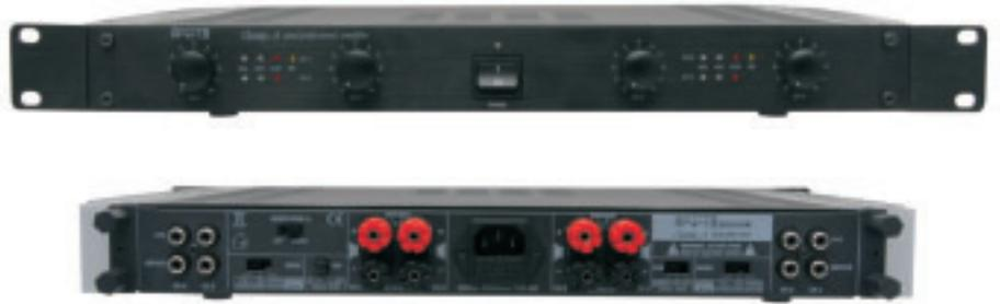
As a part of APart's revolutionary series of convection cooled power amplifiers, Champ-4 is an amplifier without cooling fans. Its four discrete AB-class amplifiers deliver high quality musical sound, high dynamics, and high reliability - all in a one-unit 19" enclosure.
